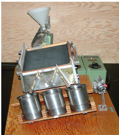
Figure 1. Vibrating deck with sample feed, sandpaper covered deck, and collection cups.
